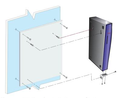
Figure 31. Wall Mounting the NetVanta 3430/NetVanta 3448
